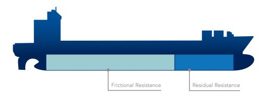
Lowering the ship resistance results in the reduction of the fuel/energy consumption and emissions. The hull optimisation generally helps to reduce the wave making and pressure resistance whereas the frictional resistance, which is dominant, considered as given and it is proportional to the wetted area. Damen Air Cavity System DACS forms stable air cavities on the flat bottom of a ship. The system has a high overall efficiency and can be used on ships for fuel consumption and emission reduction.
