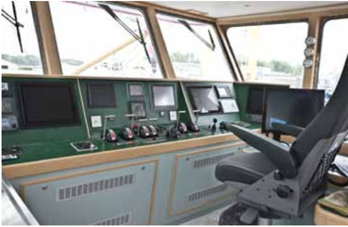
In addition to the usual controls on the bridge, also controls for all relevant fishing equipment
