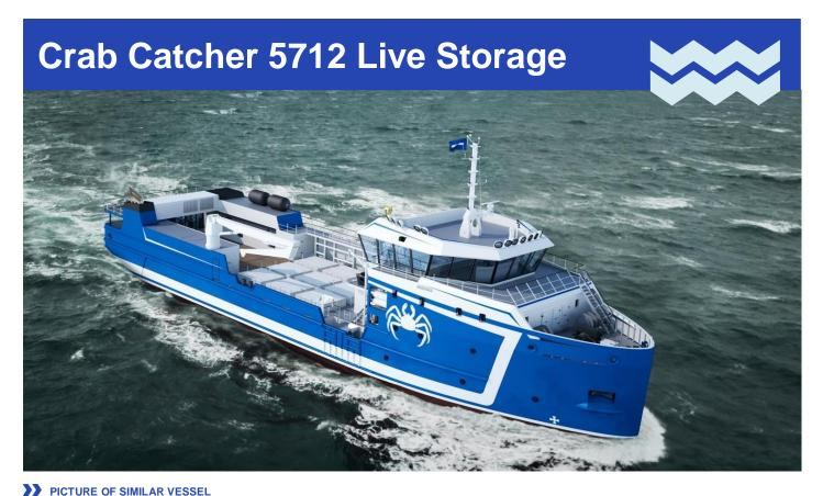
GENERAL Basic functions Crab fishing with conical pots, on-board storage in conditioned water tanks Classification
