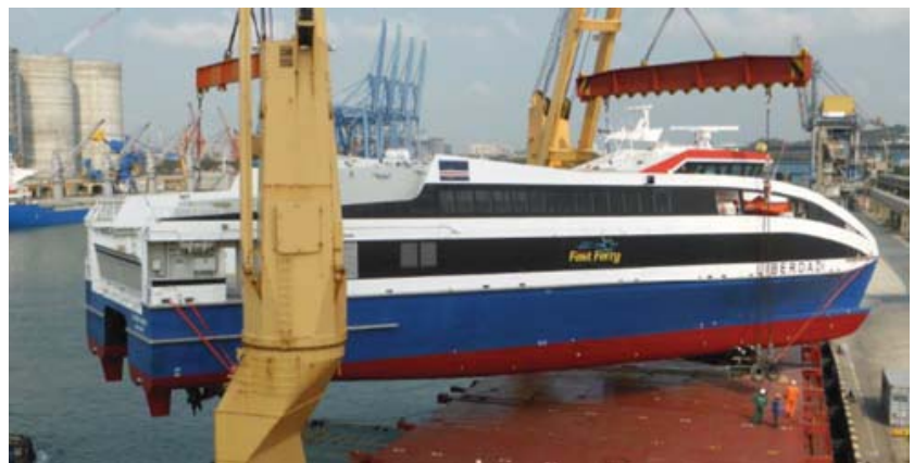
The LIBERDADI with a weight of 195 ton was lifted onboard the BBC PLATA by the two 120 ton SWL NMF cranes
