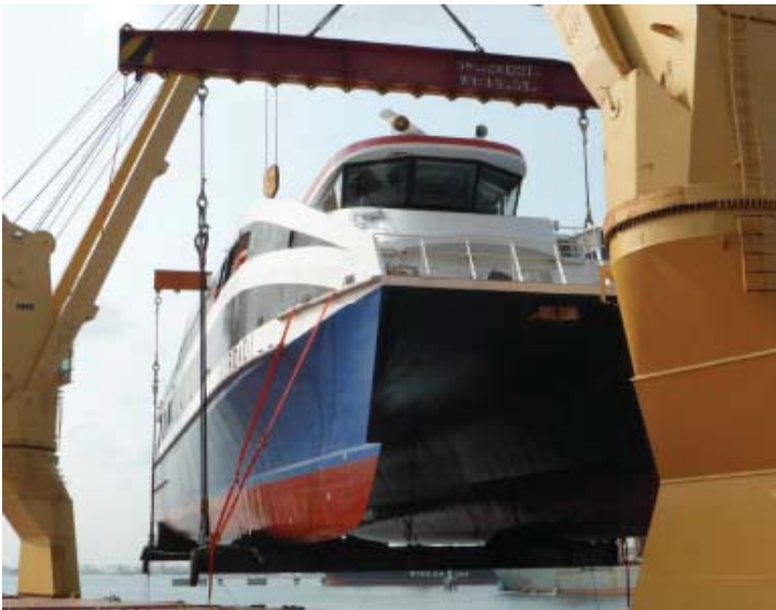
The LIBERDADI with a weight of 195 ton was lifted onboard the BBC PLATA by the two 120 ton SWL NMF cranes
