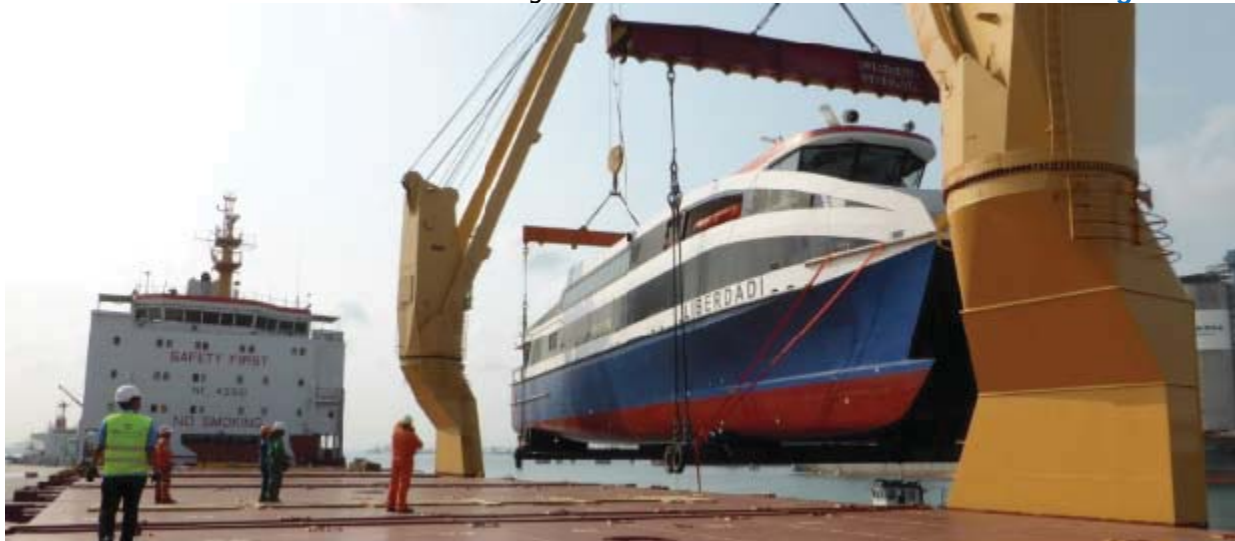
The LIBERDADI with a weight of 195 ton was lifted onboard the BBC PLATA by the two 120 ton SWL NMF cranes
