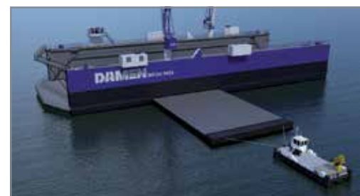
BOTTOM PONTOON IN MODULAR DRYDOCK
