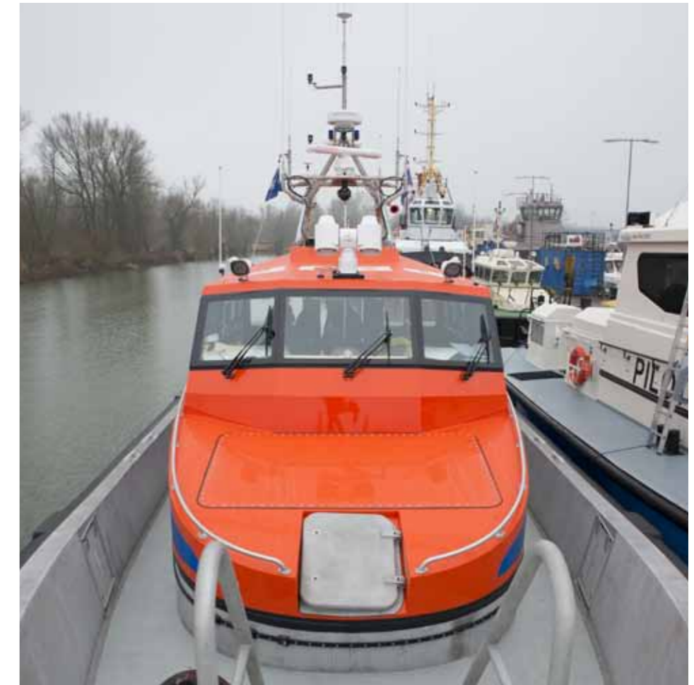
A rubber strip separates the aluminium hull from the composite deckhouse
