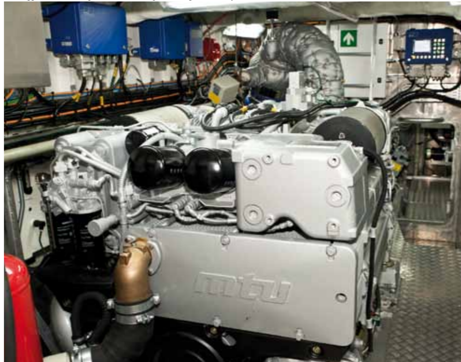
The ruggedised main engines can sustain operation upside-down for a short time
