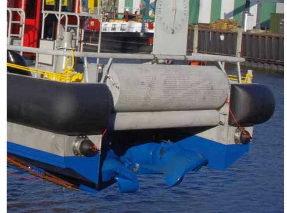
To recover survivors from the water, a basket can be hydraulically lowered
